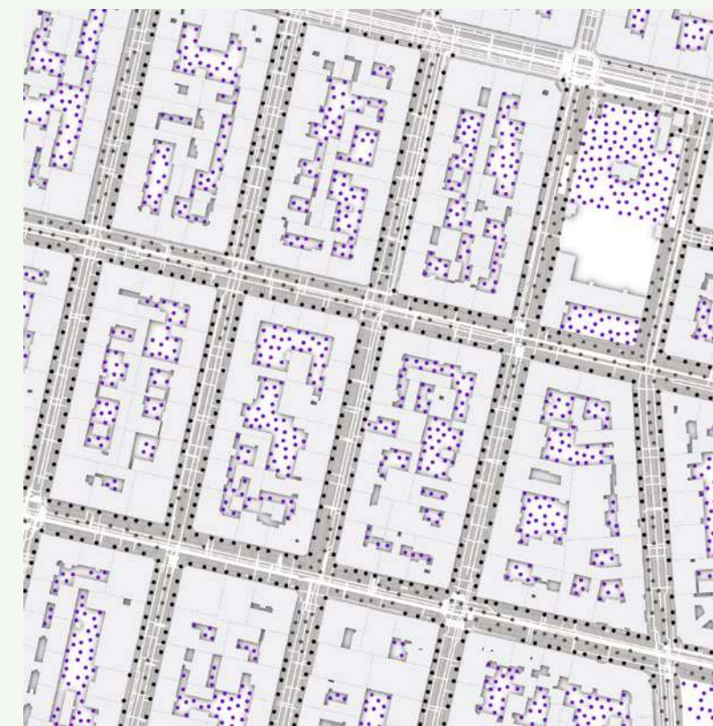
Randomly assigned locations of BHEs at given boundary conditions (e.g. minimum distances to buildings, trees, neighbouring BHEs...), source: TU Wien
