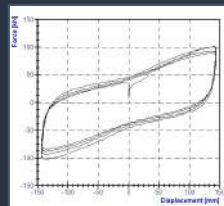
Typical hysteretic curve of a Lead Rubber Bearing
