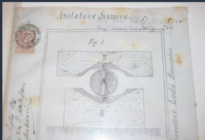
1911 – Patent of a seismic isolator by Domenico Lodà ("bearing system for buildings aimed at avoiding the transmission of seismic movements")
